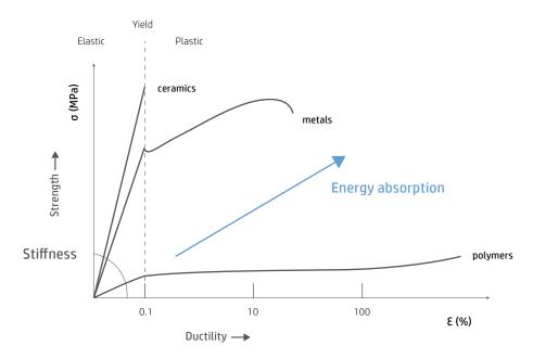
Figure 4. Comparison of polymer, metal, and ceramic materials
