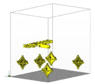
Figure 2. Dimensional test parts in half bucket part property test build. Mechanical and look and feel parts are hidden to highlight location of dimensional parts.
