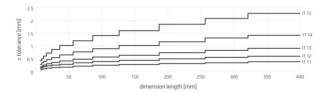
Figure 8. Tolerance range vs. dimension length
