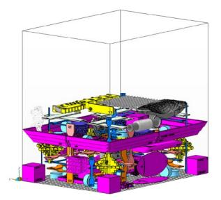
Figure 1. Half bucket part property test build. Parts are color coded by mechanical (orange/blue), dimensional (orange), and look and feel (purple/grey).
